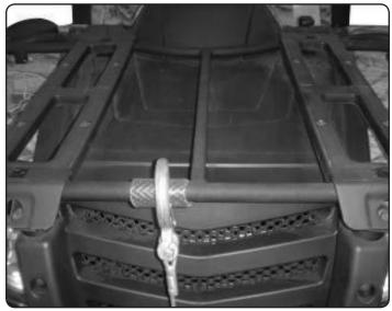
**Step 4:** Turn the control switch to the 'in' position and cautiously reel in the cable until the Snow Plow assembly begins to lift. Pay close attention to the winch, cable and clip, as well as all components and hardware of the Snow Plow assembly at this stage to ensure there are no unforeseen issues.
