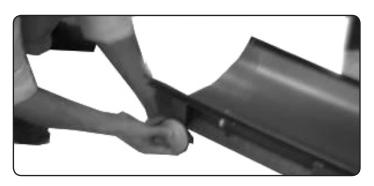
Insert the blade guides facing downwards through the feet at the base of the Plow Blade. Adjust the height of the guides to be level with the plow blade. Be sure left and right guides are at the same level. Tighten the upper and lower M12 (GB/T 6170-2000) nuts.
