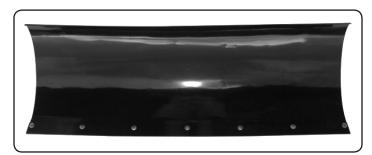
Accurately line up the Wear Blade holes to those of the Snow Plow Blade. Set it firmly and insert the 7/8/10 bolts (M1025, GB/T 794-93) and 7/8/10 nuts (M10, GB/T 6187.1-2000). Tighten.
