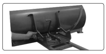
Set the Plow Blade on to the rotating plate module of the Arm Assembly, lining up the brackets. Secure each in place with a M12x1.5x38 (GB/T 5783-2000) bolt and a M12x1.5 (GB/T 6187.2-2000) nut. Tighten. Test the Plow Blade to ensure it can rotate freely.
